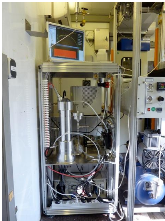
Scanning Mobility Particle Sizer, TypeSMPS-IIFT: It indicates the size and the number of particles
